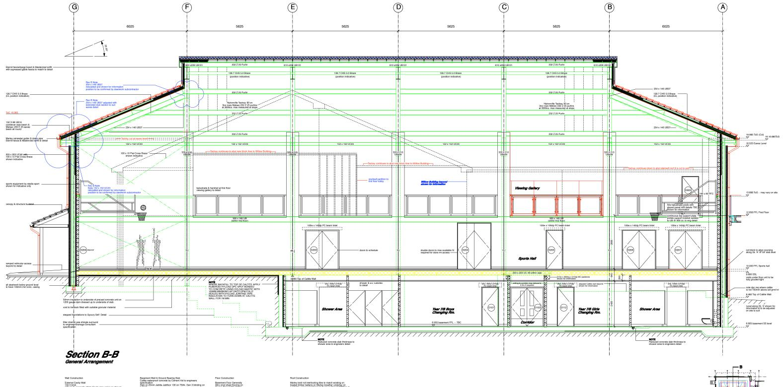
External Cavity Wall 102.5 brick 125 cavity generally (Note Cavity size varies as shown) 100 7N/mm2 block in 1:1:6 mortar
